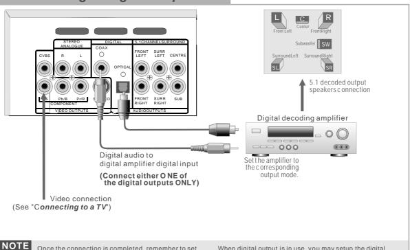
NOTE Once the connection is completed, remember to set the amplifier to the corresponding output mode. See the amplifier owner's manual.
